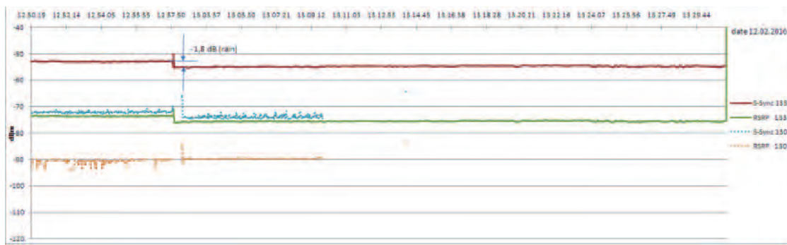
FIG. 21 Carrier power reduction for the outdoor cells upon activation of the restriction zones
